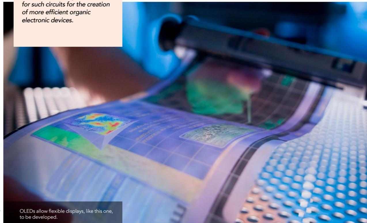
OLEDs allow flexible displays, like this one, to be developed.
