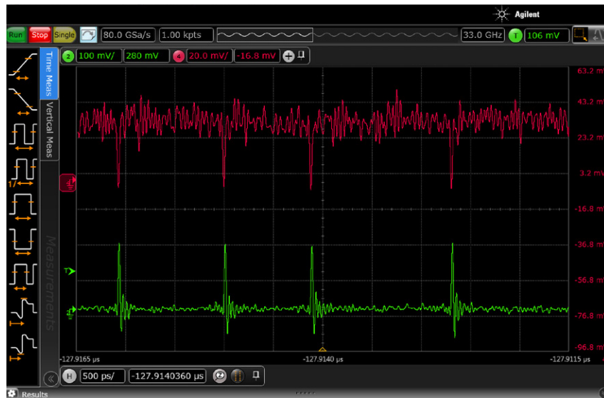
Laser emissions along two orthogonal polarisation directions of light under coherent cross-polarisation coupling condition. Upper trace: dark soliton emission. Bottom trace: bright soliton emission.
