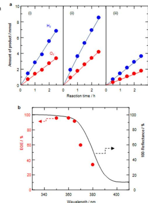
a: Time courses of H<sub>2</sub> and O<sub>2</sub> evolutions on three different photocatalysts; b: AQY(EQY) at several wavelengths.
