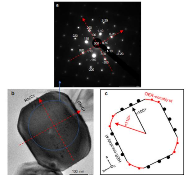
Detailed structure of a SrTiO<sub>3</sub>:Al photocatalyst particle with HER and OER co-catalysts.
