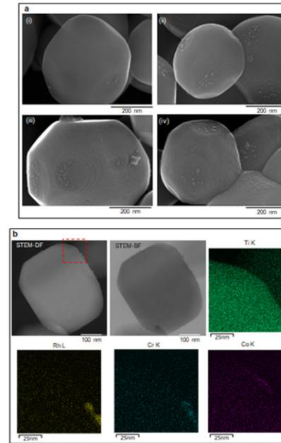
Scanning electron microscope images showing morphology of SrTiO<sub>3</sub>:Al photocatalysts with almost 100% IQY.
