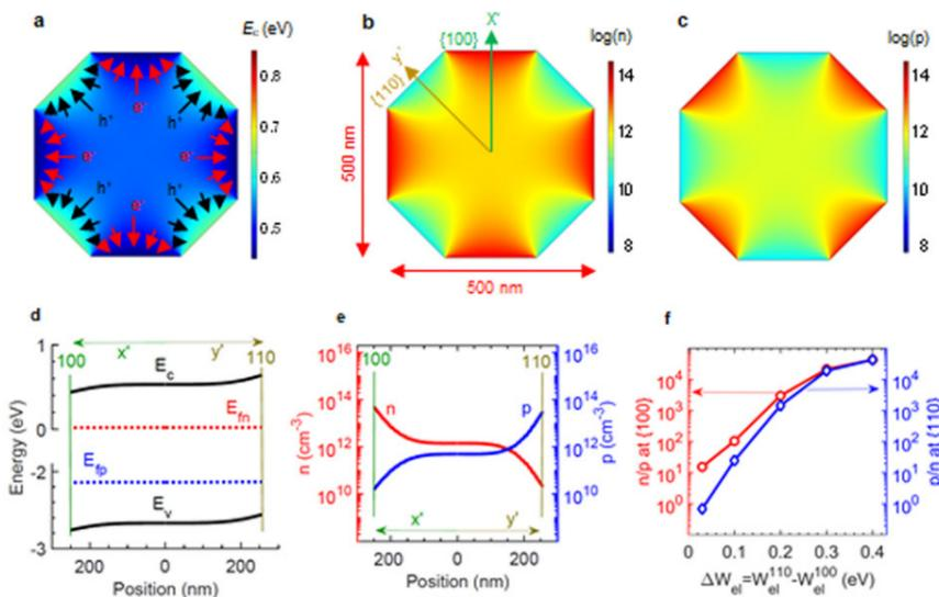
Simulated electric field, and e- and h+ distribution inside two-dimensional model structure.
