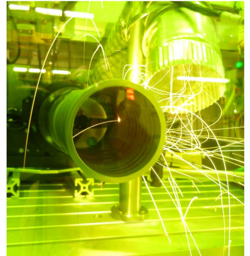
Photon momentum can accurately measure the total power in a laser beam even while it is being used to weld.
