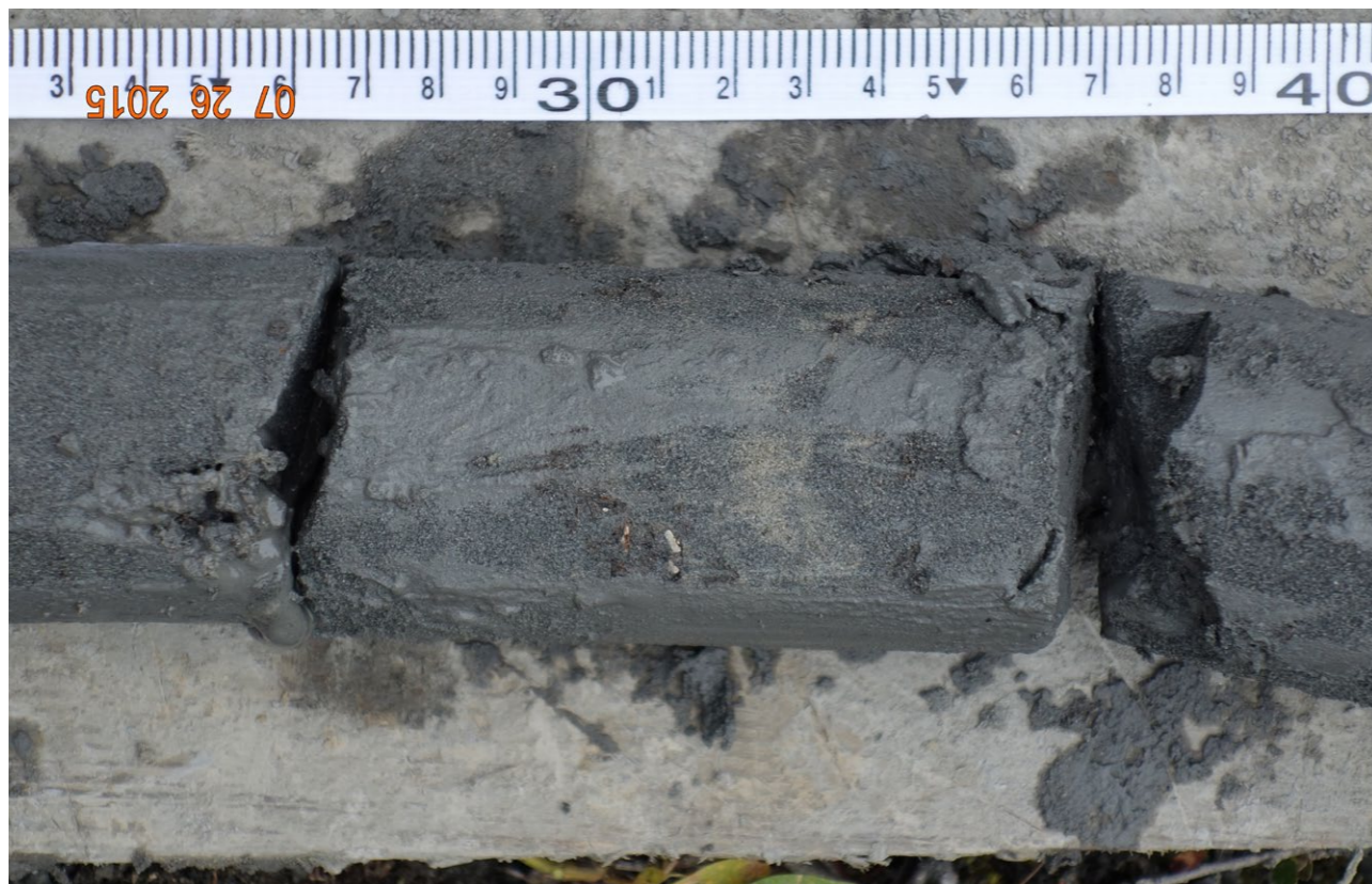
The team analysed permafrost samples collected using a rotary drill from the Kolyma–Indigirka region, Siberia.
