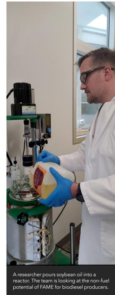
A researcher pours soybean oil into a reactor. The team is looking at the non-fuel potential of FAME for biodiesel producers.
