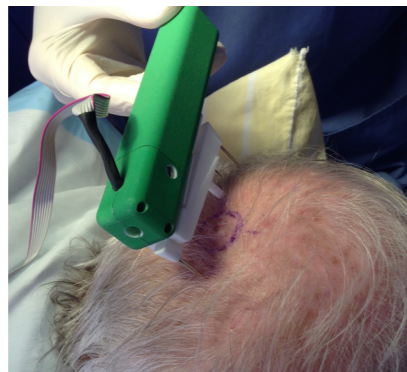
Paul is measuring tension along different directions using a specially designed tensiometer.
